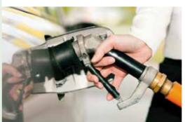
The fuel supply systems of vehicles powered by natural gas work under special pressure. They have to withstand the 200 bar under which the fuel natural gas is stored in the tank – and in addition to this remain leakproof for the whole life of a vehicle. So it goes without saying that every component used in the gas unit has to meet the highest production standards.
