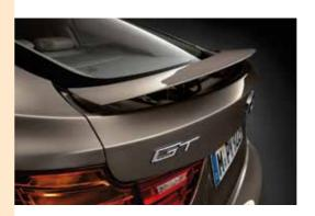
It's reserved and it's not so easy to lure it out of its hideaway: the extendable rear spoiler of the BMW 3er GT only appears when it gets up to a speed of 110 km/h. A professional pretreatment and coating is essential for its successful appearance – even after years of use. After all, the rear wing of galvanized sheet steel is exposed to strong physical influences: its surface is eaten away by spray water, ice, salt, or the impact of flying stones.
